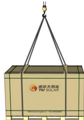
Figure 5 Schematic diagram of Module lifting
